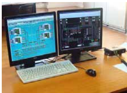
To control the entire terminal a two-screen workstation was installed running SCADA Reliance
